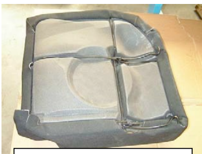
The XLPE foam is inserted into the seat frame
