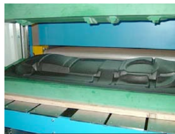
The foam roll is then heated and formed on the male mold
