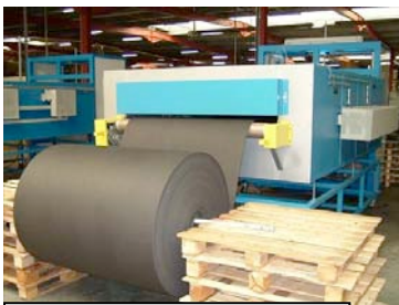
XLPE foam roll fed into the thermoforming machine from the rear
