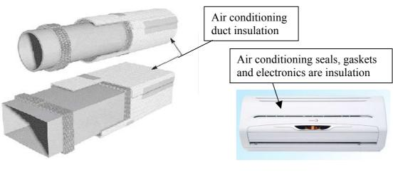
Foam Sheaths for A/C piping – connecting the wall unit to the outdoor heat exchanger
