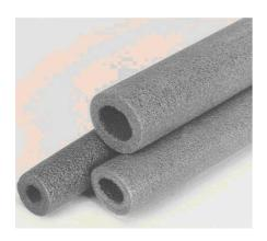
F 1.1FRIZ "Deca- DBE-Free" Fire retardant foams for pipe and Air conditioning duct insulation (18kg/m³/1.1PCF) Classified as UL94 HF-1 and (GA20FRF) ASTM E84 25/50
